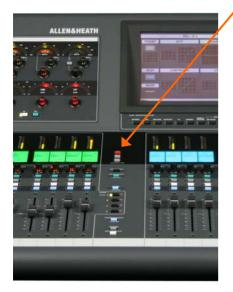
**COPY** / **PASTE** / **RESET keys** These functions are protected from accidental operation. Pressing one of these keys by itself does nothing. The edit function is actioned only if the key is first held down and then a **SEL** or **MIX** key elsewhere on the surface is pressed while it is held.
